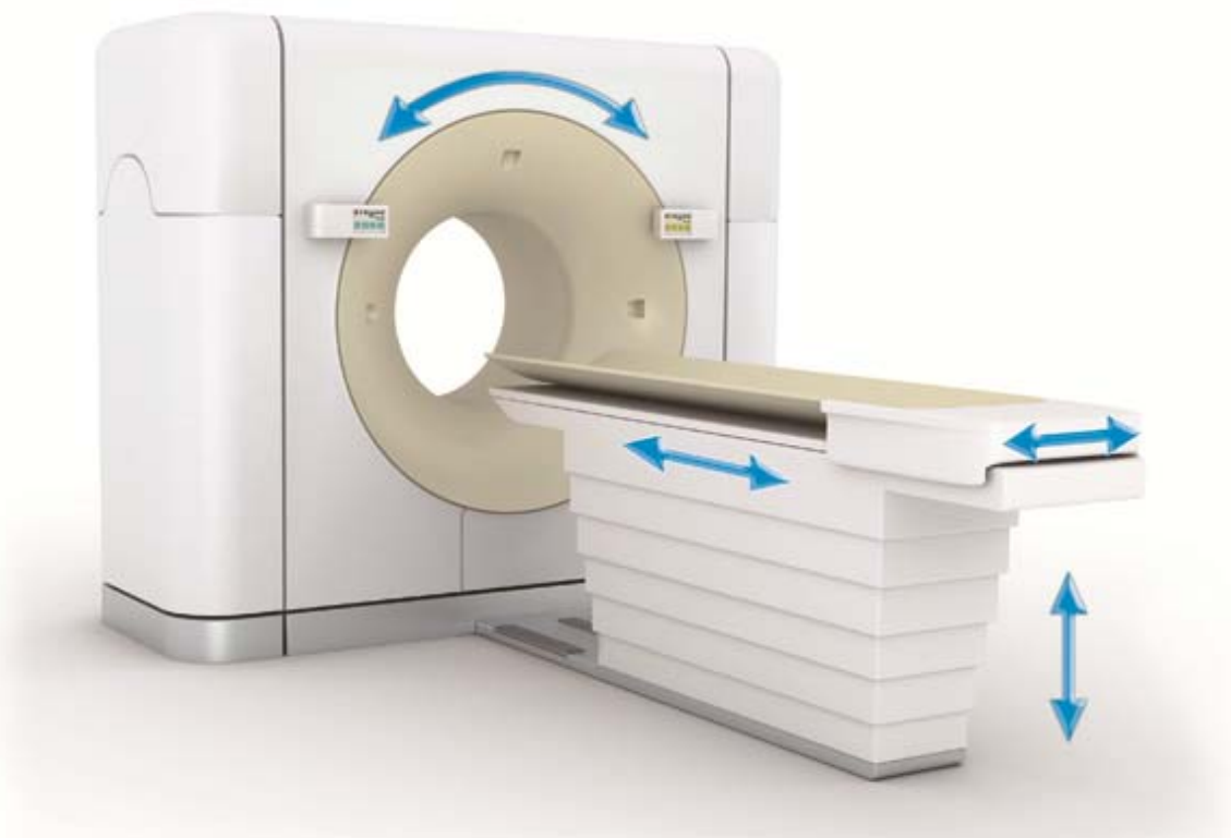
Fig. 15: Rotational and length measurement in a computer tomography unit
