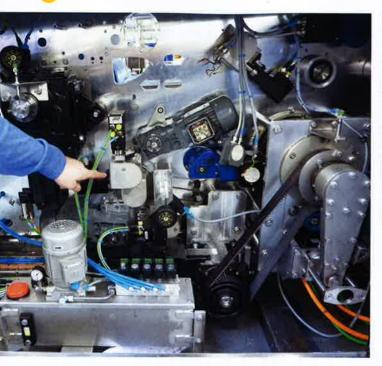
selected, all actuators go to the new position and production can be continued immediately. In addition to the drastic reduction of set-up times, another important advantage is the precise reproducibility of the baking results.
