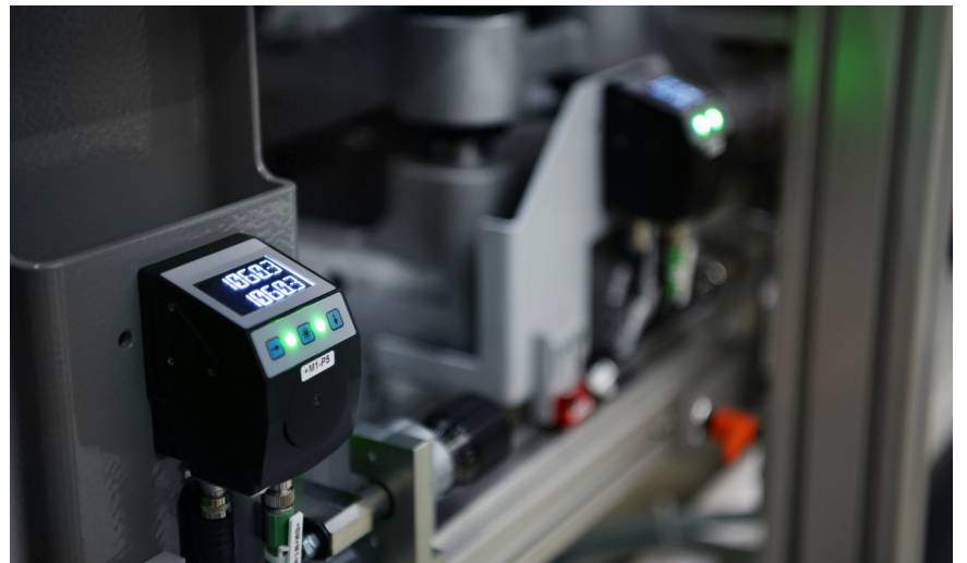
The green LEDs of the SIKO AP10S position indicator clearly indicate that the stations on the Z.PACK blister machine are set up correctly and the packaging process can continue.
