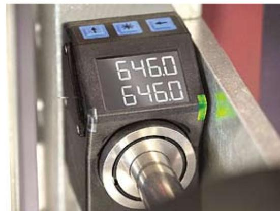
The SIKO position indicator AP05 with green status LEDs shows a correct machine setting. (Photo © SOMIC)
